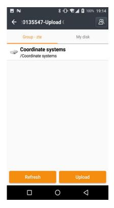
Click "From cloud" to enter the coordinate system folder in the cloud disk, and click "download" to download the coordinate system file and save it to the coordinate system. You can view it by creating a new coordinate system and search the coordinate system file by keyword.
