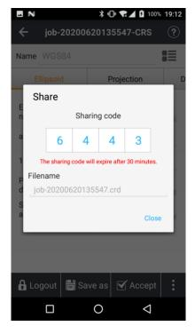
Click "Load" enter the 4-digit correct sharing code, click "get" to obtain the shared coordinate system parameters, "open" becomes optional, and click "open" to open the obtained coordinate system parameters.
