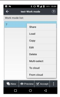
Select the saved working mode and click "share " to generate a 4-digit sharing code, it will display the name of the transferred file. The sharing code is valid for 30 minutes.
